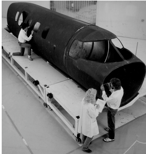
Figure 2 Beech Filament Wound Starship Fuselage Fibertek Photo
